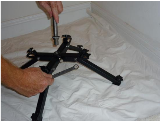
Figure 2.7-Removing Spindle from Quad Pod
