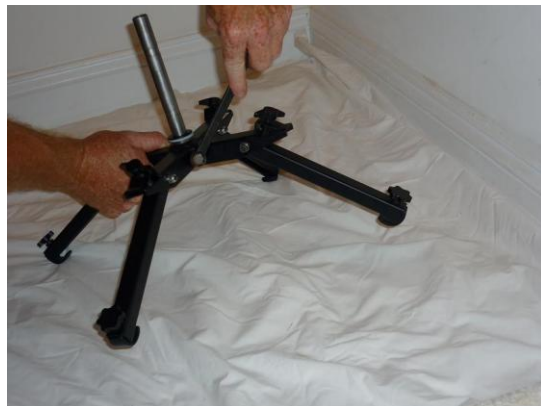
Figure 2.6-Loosening Spindle anchor bolt on Quad Pod
