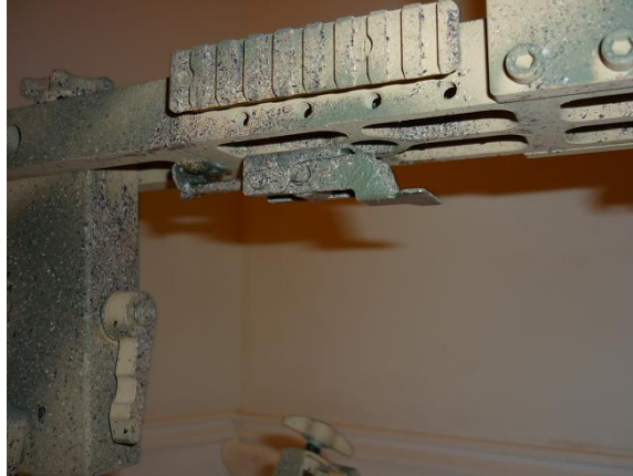
Figure 2.14- Lower Binding Latch/Head
