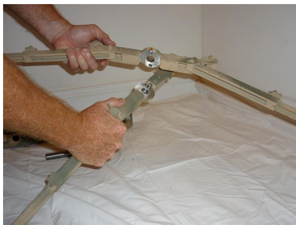
Figure 2.13- Quad Pod intersecting guide pins
