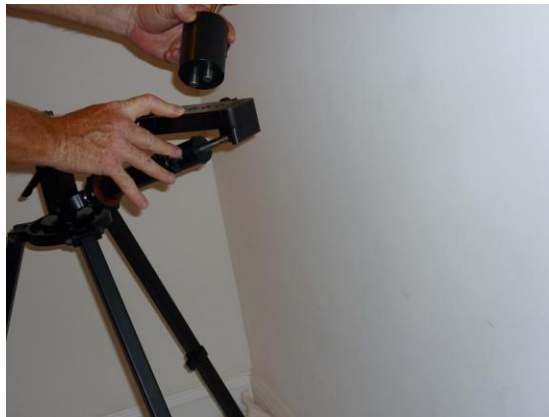
Figure 2.3-Yoke Arm Extender Removal
