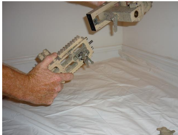
Figure 2.15- Guide Pins and Anchor Stud
